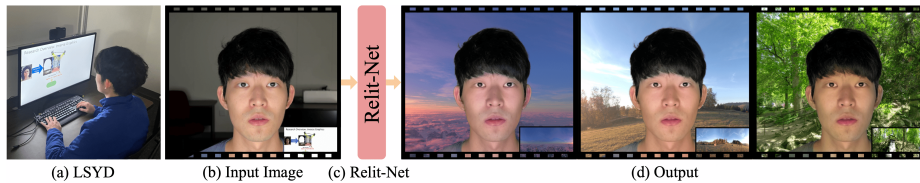
Fig. 1. We learn a personalized relighting algorithm that generates temporally consistent and high-quality portrait videos under different lighting. We train the network using recordings of users watching YouTube on a monitor, thereby creating a Light Stage at Your Desk (LSYD). We project a portion of the LDR environment map with a 180^\circ FoV as the monitor light, while a portion of the remaining 90^\circ FoV is mapped as the background. We can achieve a harmonization effect with the virtual background.
